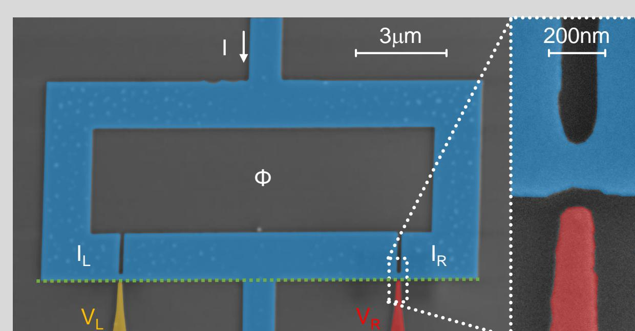
The SQUID is realized with a single-step electron beam lithography and 30 nm-thick evaporation of Titanium. The two junctions consist in two constrictions (Dayem bridges) 150 nm x 150 nm. Each junction is gated by a correspondent electrode, distant 30 nm and 50 nm from the right and left junction
