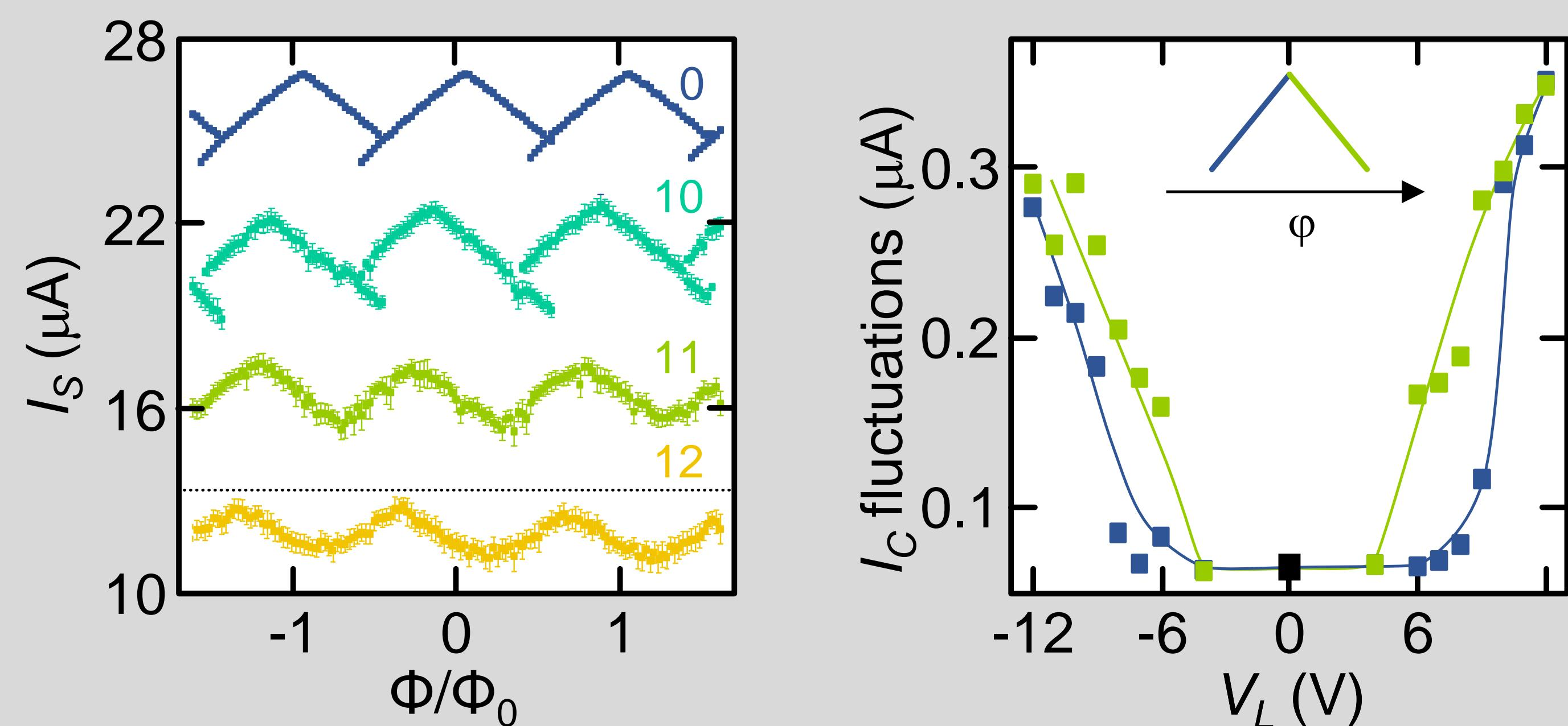
At higher voltages, the switching current interferes even below the single junction critical current. This effect cannot be explained within a SQUID model where the single junction critical current is suppressed by the electric field. In this case, indeed, a switching current independent on the flux (due to the ungated junction) is expected.
