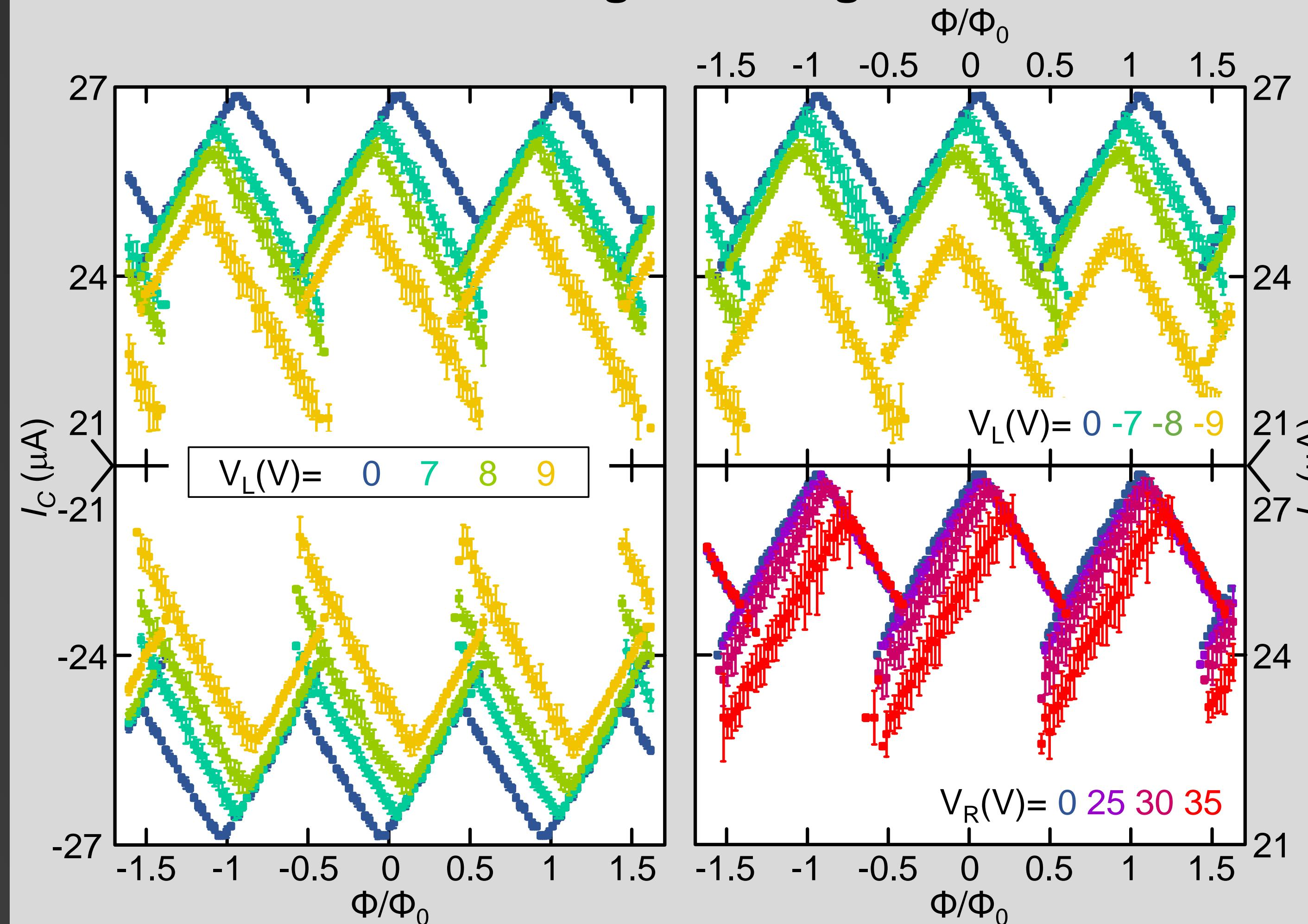
**We demonstrated an unconventional presence of field-effect, affecting the switching current characteristic versus the magnetic flux  $I_S(\Phi)$ .**
