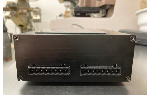
Pulse ports, 2x8-pin euro-style
